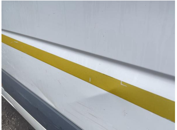
10: Door nsr Dented With Paint Damage
