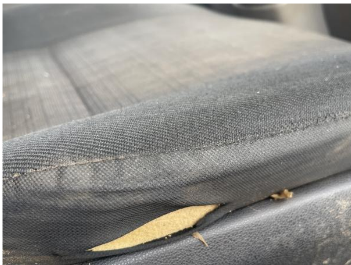
1: Seat Base Cover osf Torn Over 3mm
