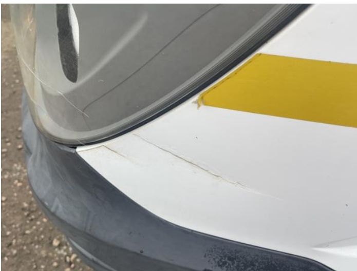
13: Wing nsf Dented With Paint Damage
