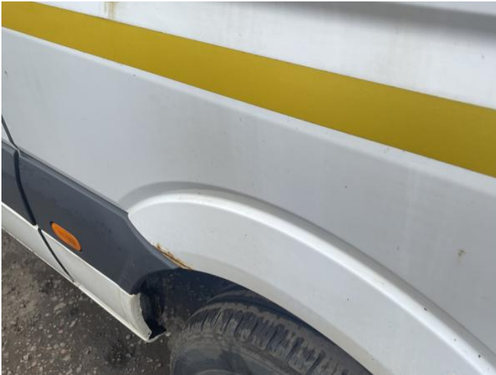
9: Qtr Panel nsr Rusted Over 5mm
