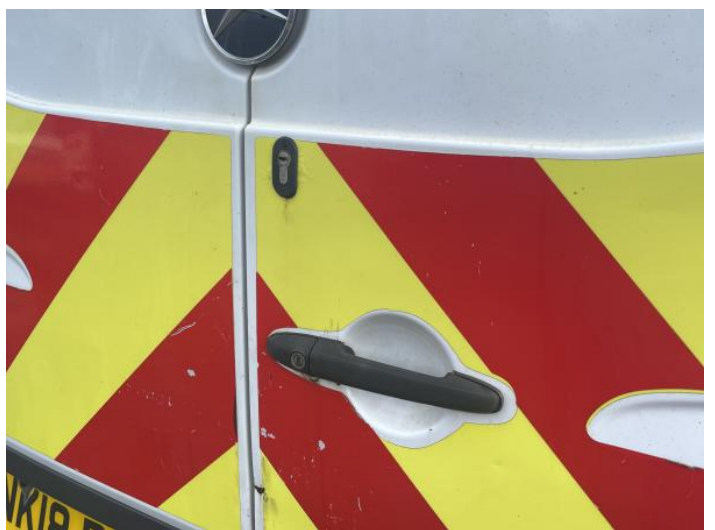
8: Tailgate Dented With Paint Damage
