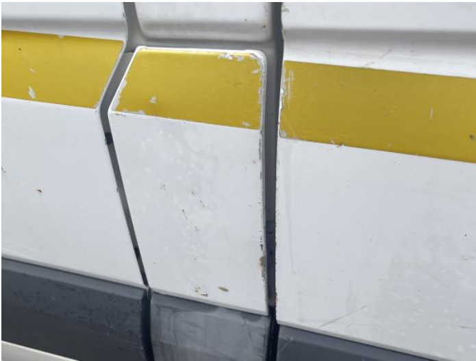
11: B Post ns Rusted Over 5mm
