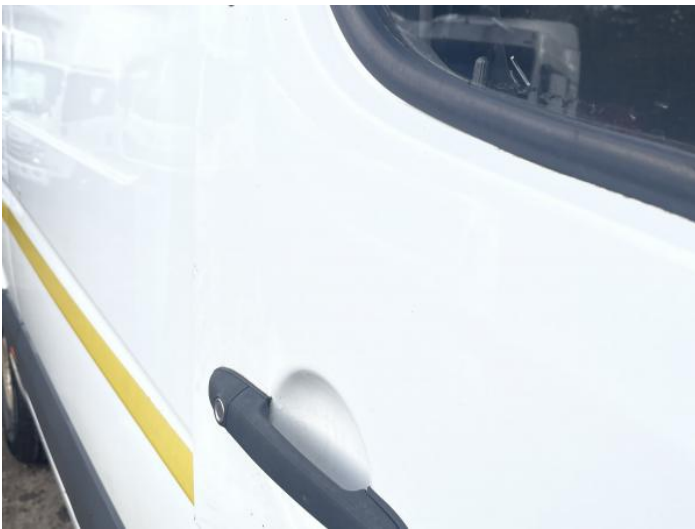
5: Door osf Dented Over 30mm
