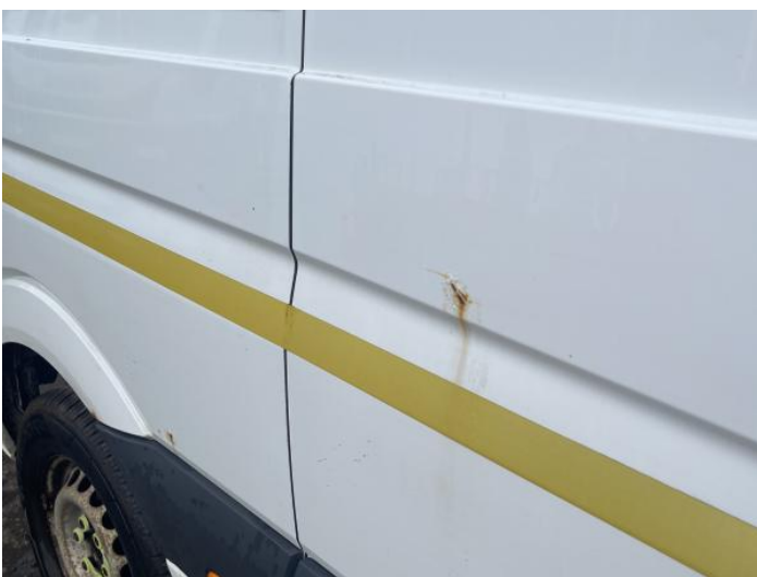
7: Qtr Panel osr Rusted Over 5mm
