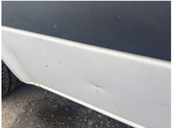
12: Door nsf Dented With Paint Damage
