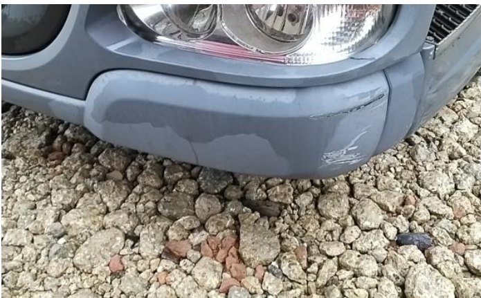
3: Bumper Front Moulding Scuffed (Unpainted) UpTo 100mm
