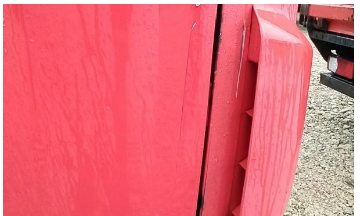
12: Panel Rear Scratched Over 25mm Thru Paint
