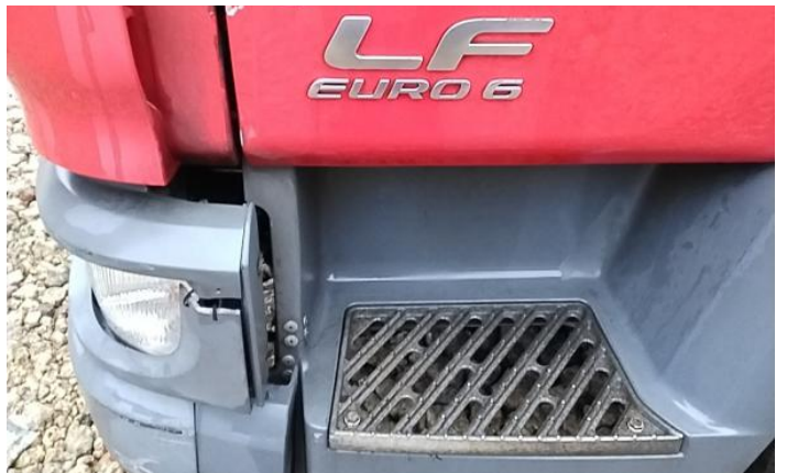
6: Bumper Front Moulding Scuffed (Unpainted) Over 100mm
